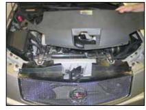
3. Remove the radiator cover from the vehicle.
