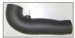
20. Install the crank case vent fitting into the K&N® intake tube as shown.
