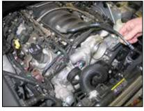
7. Remove the factory crank case vent hose from the valve cover.
