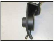
16. Assemble the mass air sensor and filter adapter with the provided gaskets onto the heat shield as shown using the provided hardware.
