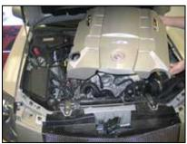
6. Lift up the engine cover to dislodge it from the mounting grommets and then remove the cover from the vehicle.
