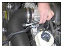
23. Install the provided crank case vent hose onto the valve cover and then connect the open end to the vent fitting on the K&N® intake tube.
