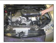
5. Loosen the hose clamps which secure the intake tube to the throttle body and air filter, then remove the intake tube from the vehicle as shown.
