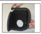
13. Install the edge trim onto the heat shield as shown.
