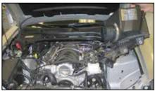
10. Remove the air box assembly from the vehicle. NOTE: K&N Engineering, Inc., recommends that customers do not discard factory air intake.
