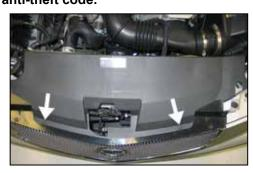
2. Release the two radiator cover retaining pins.
