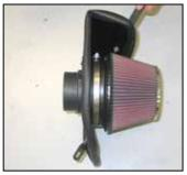
17. Install the K&N® air filter onto the filter adapter and secure with the provided hose clamp.
