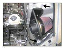
18. Install the heat shield assembly into the engine compartment and secure with the provided hardware.
