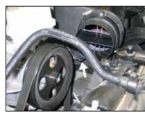
8. Disconnect the mass air sensor electrical connection.
